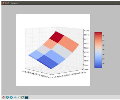
The first model had a length of 1 meter and a width of 0.5 meters. To maximize the Rover's stability in both the x and y, 0.75 meters was selected. Cost and practicality are limiting factors in making the rover any larger. For the target applications, the general size of a yard lawn mow used as a guiding principle. This improved the combined static stability as the table below shows:
